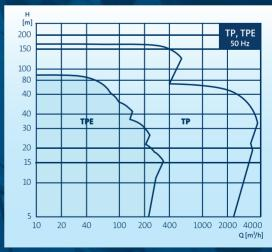
The curve shows the performance area of Grundfos in-line pumps. The shaded area shows the performance area of pumps with integrated frequency converters (TPE pumps)
