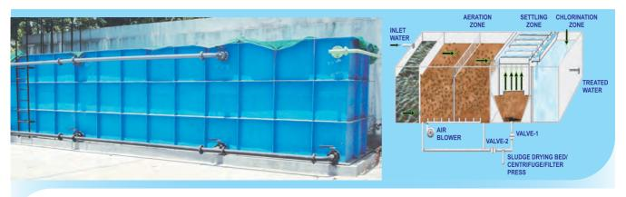
INDION Fluidised Media Reactor (FMR) is designed as a single tank unit, incorporating a bar screen chamber, specially developed synthetic media to facilitate attached growth process, oxygen transfer through diffused membrane aeration, a lamella settler and a chlorine contact tank for disinfection.
